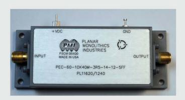
PMI Model No. PEC-60-10K40M-3R5-14-12-SFF is a low noise amplifier that operates from 10kHz to 40MHz. This amplifier provides over 60dB of gain and offers a low noise figure of 3.5dB maximum. The output power at 1dB gain compression is +14dBm minimum. This amplifier operates from a single +12V or +15V DC supply. The housing measures 3.07" x 1.18" x 0.5".
